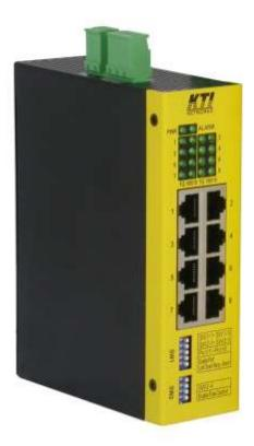
The switch provides eight 10/100/1000Mbps copper ports for connections to Ethernet, Fast Ethernet or Gigabit Ethernet devices. With the featured auto-negotiation function, the switch can detect and configure the connection speed and duplex automatically. The switch also provides auto MDI/MDI-X function, which can detect the connected cable and switch the transmission wire pair and receiving pair automatically. This auto-crossover function can simplify the type of network cables used.
