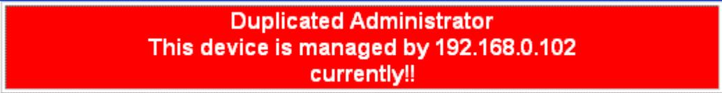
A new connection will be accepted when the current user logout successfully or auto logout by the device due to no access for time out of 3 minutes. System Configuration is displayed after a successful login.
