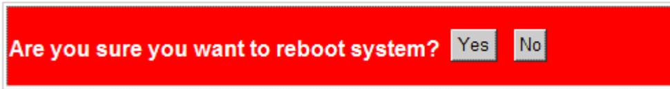
This menu is used to reboot the device remotely with current configuration. Starting this menu will make your current http connection lost. You must rebuild the connection to perform any management operation to the unit.
