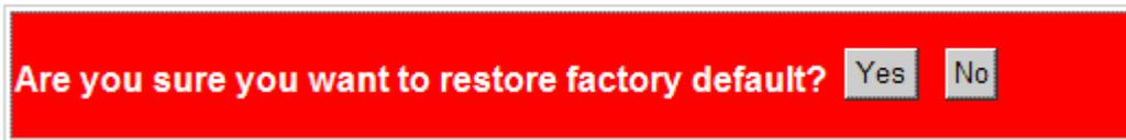
This menu is used to restore all settings of the device unit with factory default values. Note that this menu might change the current IP address of the device and make your current http connection lost.
