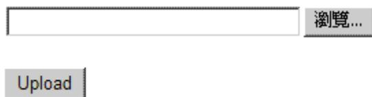
This menu is used to perform in-band firmware (software) upgrade. Enter the path and file name of new firmware image file for uploading.
