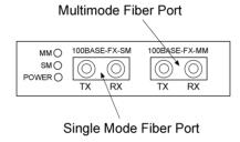
The multimode fiber port is used for a duplex multimode fiber cable connection and single mode fiber port is used for a duplex single mode fiber cable connection.
