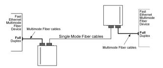
**Important rule:** When a connection is established, make sure the devices located at both ends of the path are configured and operated using the same duplex mode and the maximum distance must comply with IEEE 802.3u specifications.
