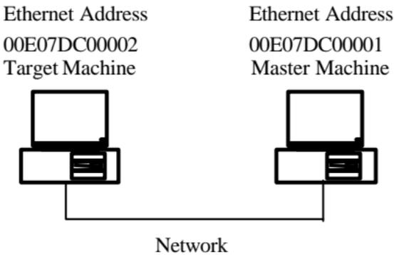
**Master Machine:** Master machine sends magic packet or Wake up frame through the network.
