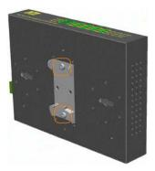
Mount the device on a Din-rail.
