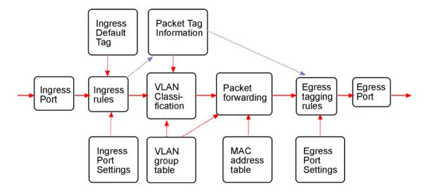
The following sections describe the VLAN processes and **Advanced VLAN mode** settings provided by the switch. A global setting means the setting is applied to all ports of the switch. A per port setting means each port can be configured for the setting respectively.
