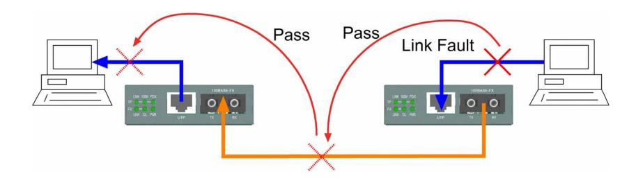
The device at local end is able to detect link fault at the remote copper connection.
