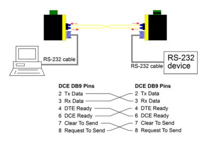
The converter converts all signals of the COM port of the PC to optical signals and sends to the other converter far apart over fiber cable.
