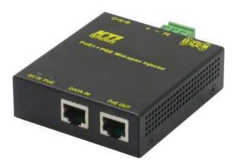
Power over Ethernet provides a way for Ethernet network devices to be powered by UTP cables, including Cat.5, 5e, and 6 rather than by separate power cords. The device is a mid-span injector that can deliver output power supporting proprietary PoE++ 90W Type 4 PDs, 802.3at Type 2 high-power PDs, and 802.3af Type 1 PDs. The injector supports both Fast Ethernet connection and Gigabit Ethernet connection.
