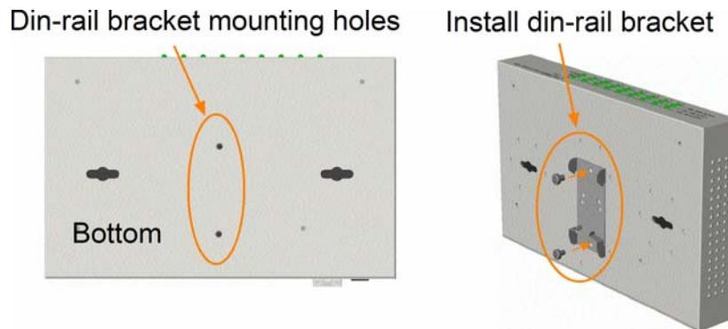
2. Mount the units on a din-rail chassis
