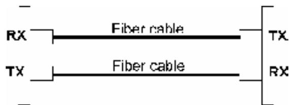
Make sure the Rx-to-Tx connection rule is followed on the both ends of the fiber cable.
