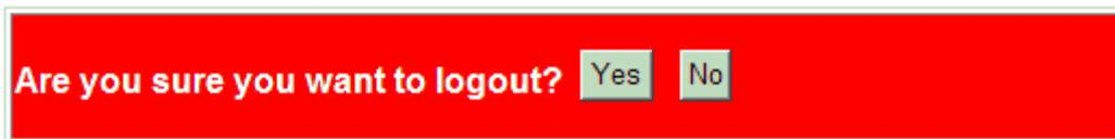
This menu is used to perform a logout from the switch management. If current user does not perform any management operation over 3 minutes, the switch will execute an auto logout and abort the current connection.
