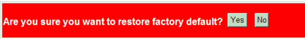
This menu is used to restore all settings of the switch unit with factory default values except current IP configuration and Management VLAN configuration.
