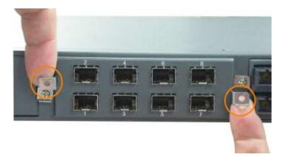
4. Remove the module from the slot.
