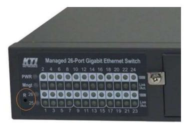
The reset button is used to perform a reset to the switch. It is not used in normal cases and can be used for diagnostic purpose. If any network hanging problem is suspected, it is useful to push the button to reset the switch without turning off the power. Check whether the network is recovered.
