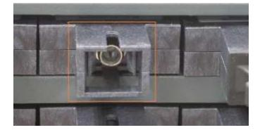
A Bi-Di port supports single fiber connection. It uses different optical wavelengths for transmission and receiving individually as figure illustrated below:
