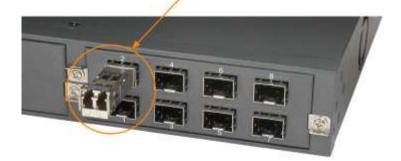
3. Until the SFP transceiver is seated securely in the slot, place the bail in lock position.
