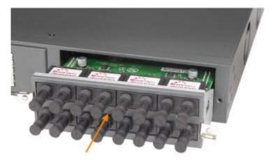
3. Screw the module on the front panel of the base chassis securely. Screw the module into the base
