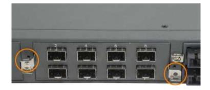
3. Use the brackets as handles to pull the module out from the module slot connector.
