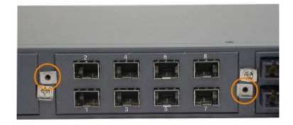
2. Loosen two screw brackets and pull them out as shown below:
