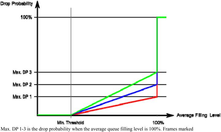
Max. DP 1-3 is the drop probability when the average queue filling level is 100%. Frames marked with Drop Precedence Level 0 are never dropped. Min. Threshold is the average queue filling level where the queues randomly start dropping frames. The drop probability for frames marked with Drop Precedence Level n increases linearly from zero (at Min. Threshold average queue filling level) to Max. DP n (at 100% average queue filling level).
