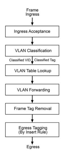
Each incoming frame on the ingress port passes "Ingress Acceptance" process first for filtering accepted frames and discarding others. Then, the frame gets into "VLAN Classification" process for getting Classified VLAN and classified tag. The "Classified VLAN" is used for VLAN table lookup and VLAN bridging operation. The "Classified tag" is used for tag insertion for egress tagging is required.
