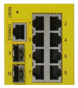
The connector designed for the console port is RJ-45.
