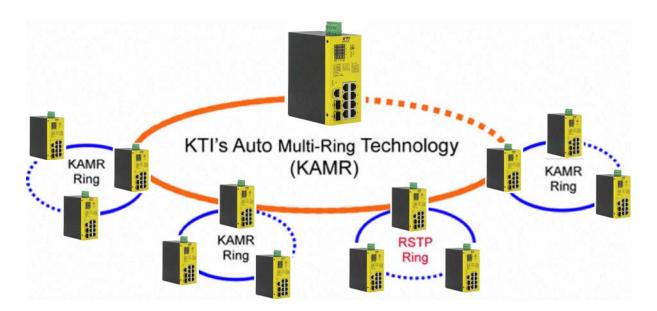
The following figure shows one switch is configured to support three redundant rings and one RSTP ring at the same time.
