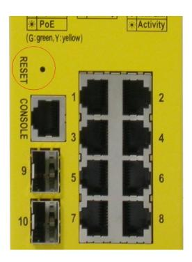
The button can also be used to restore the software configuration settings to factory default values.
