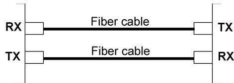
Make sure the Rx-to-Tx connection rule is followed on the both ends of the fiber cable.
