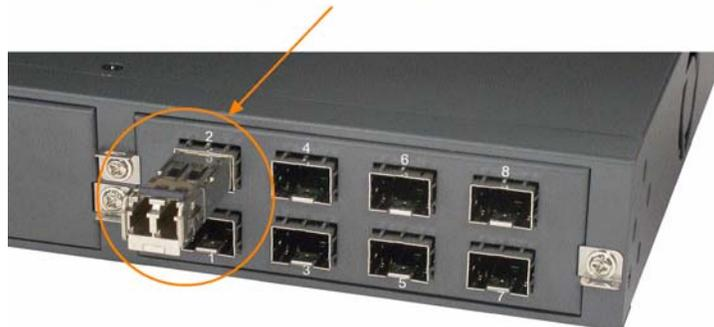
3. Until the SFP transceiver is seated securely in the slot, place the bail in lock position.
