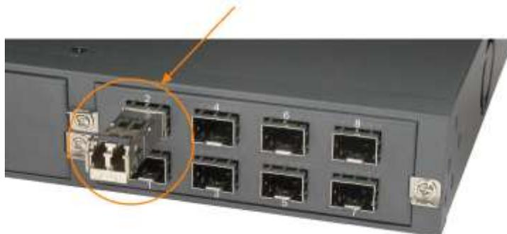
3. Until the SFP transceiver is seated securely in the slot, place the bail in lock position.
