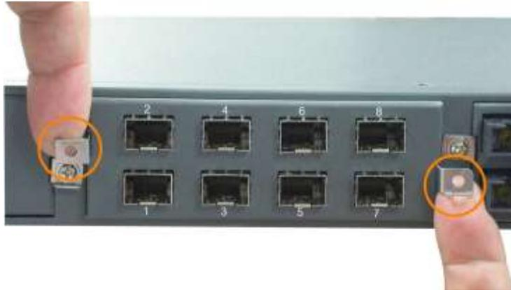
4. Remove the module from the slot.
