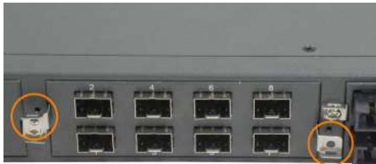
3. Use the brackets as handles to pull the module out from the module slot connector.
