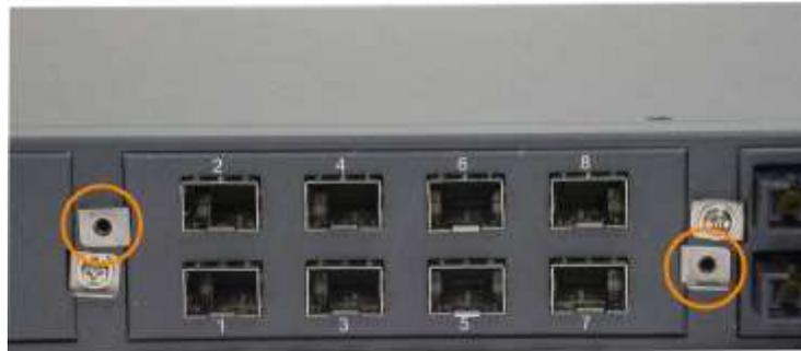
2. Loosen two screw brackets and pull them out as shown below:
