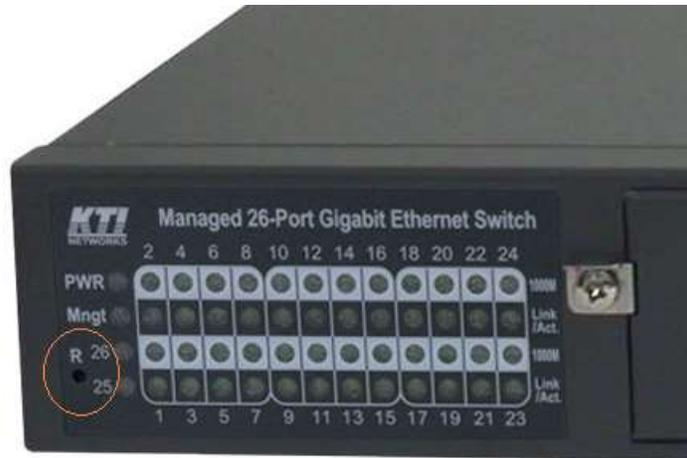
The reset button is used to perform a reset to the switch. It is not used in normal cases and can be used for diagnostic purpose. If any network hanging problem is suspected, it is useful to push the button to reset the switch without turning off the power. Check whether the network is recovered.
