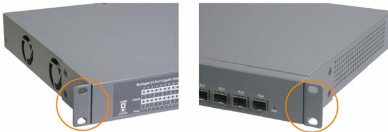
Install rack mounting brackets
